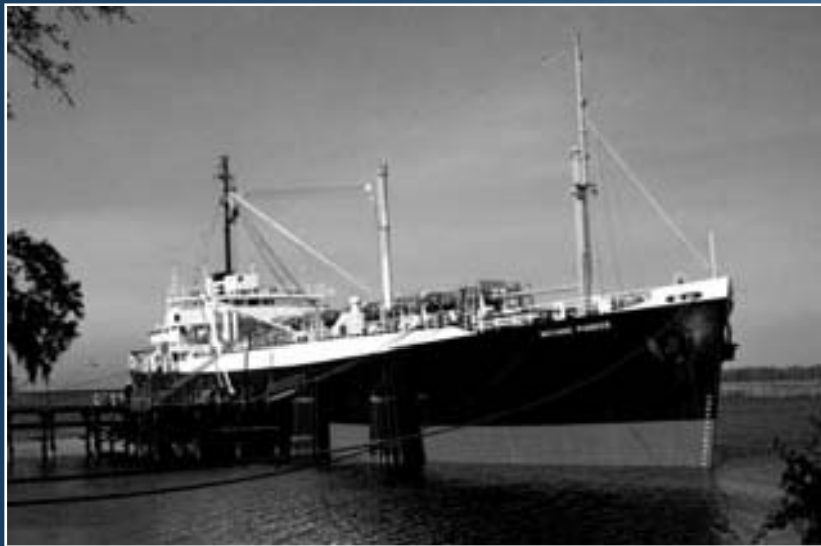
British Gas Canvey Island LNG Terminal January 1959: A World First: ‘Methane Pioneer’ 5,000 m 3
