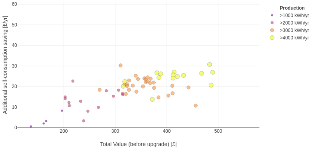
Figure D-1: Self-consumption savings due to BESS size increase: all 5kWh to 7.5kWh (counterfactual)
