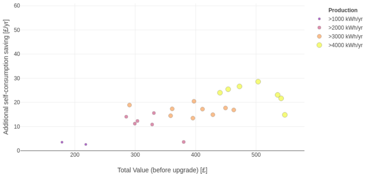
Figure D-2: Self-consumption savings due to BESS size increase: all 7.5kWh to 10kWh (counterfactual)
